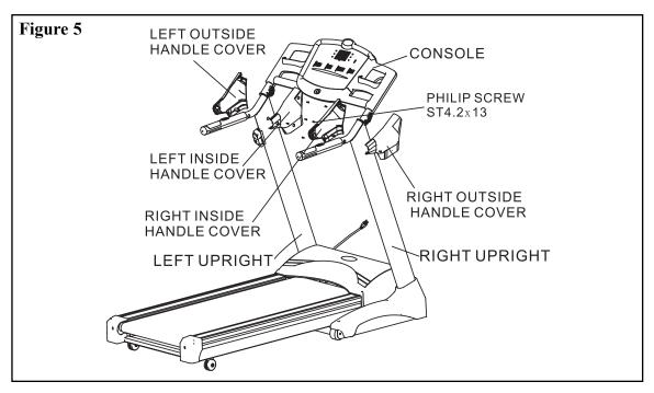
6. Tighten all allen bolts (Qty. 8) installed in Step 3. **Note:** Move the fenders up to access the allen bolts. Next, attach both left and right fenders to base using philip screw ST4.2x13 (Qty. 2) and philip screw M6x12 (Qty. 2).
